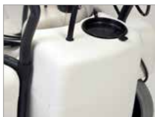
EXTERNAL DETERGENT TANK
