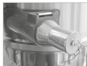
RESISTANT FRAMEWORK AND INLET PLUG FOR SAFE TRANSFER
