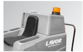
Reverse lighting and acoustic warning system
