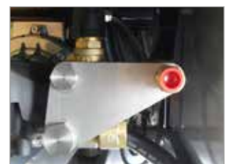
BY-PASS VALVE IS PROVIDED WITH 1 HOLDING METAL PLATE IN ORDER TO PROTECT IT FROM MECHANICAL STRESS
