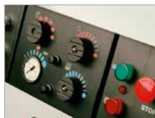
CONTROL PANEL PROVIDED WITH EMERGENCY SHUTDOWN
