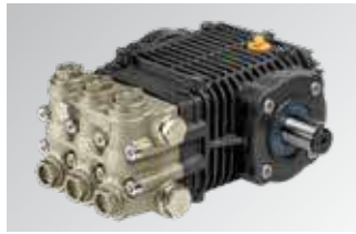
New CL 6.0 self-priming three-piston integral ceramic pump, tapered roller bearings, double oil viewer, nickel-plated brass head and high temperature water seals
