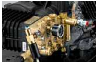
New CL 6.0 self-priming pump with three pistons in integral ceramic, double oil viewer and brass head. Speed reducer between motor and pump. New flanged pressure regulating valve L3.1, internal passages resized to ensure correct operation even in high operating flow conditions
